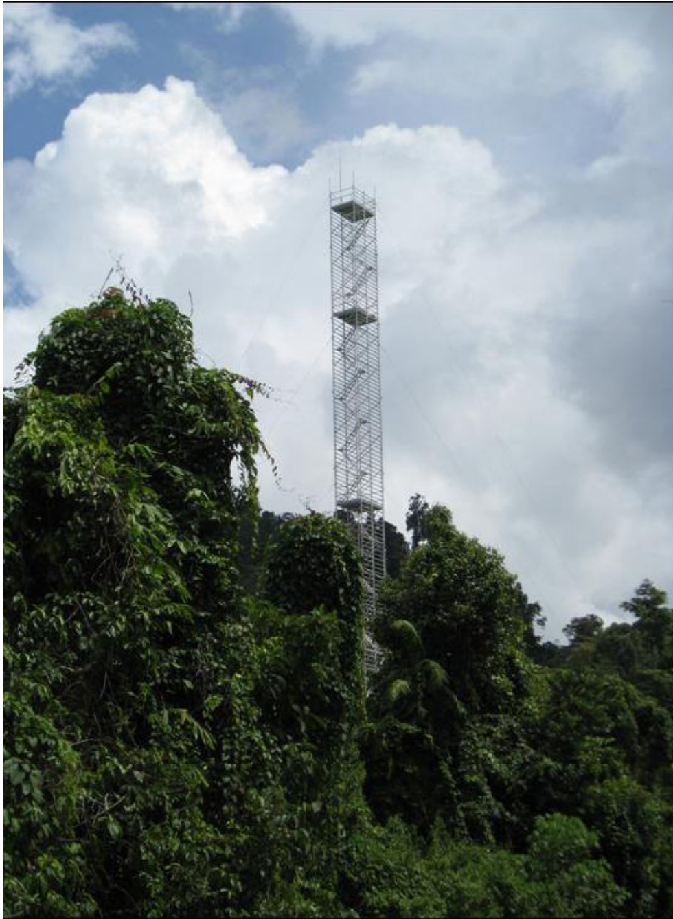
Figure 3 Carbon flux tower in the SAFE experimental area. This 50 m-high tower is situated in an area of forest that will be converted to oil palm during 2012. By recording detailed measures of carbon flux over this period, the impact of the establishment of a new plantation on an area's carbon balance can be measured
